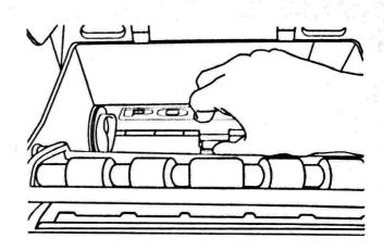
Slide and lift the battery compartment lid, insert 4 LR20 (size D, mono cells) alkaline batteries with correct polarity, and close the battery compartment lid.
