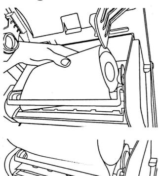
When the roll reaches the edge of paper holders, it can be placed in the cabinet for reserve roll without interrupting paper feed.
