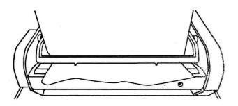
Release the rocker and close the hood. The dispenser will feed the paper automatically.
