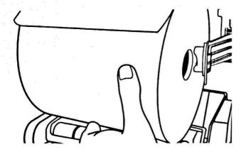
Insert the paper towel roll between paper holders and make the core fit properly into holder arms.
